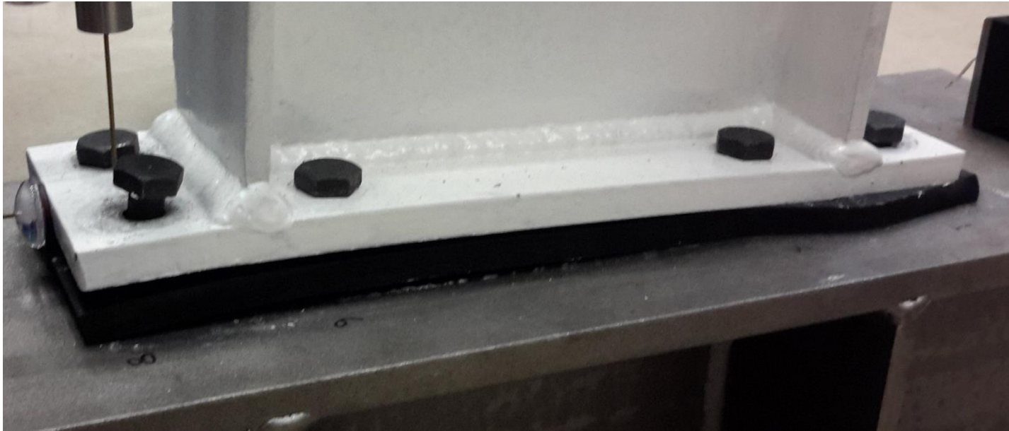
0.5 in. neoprene pad test at failure
