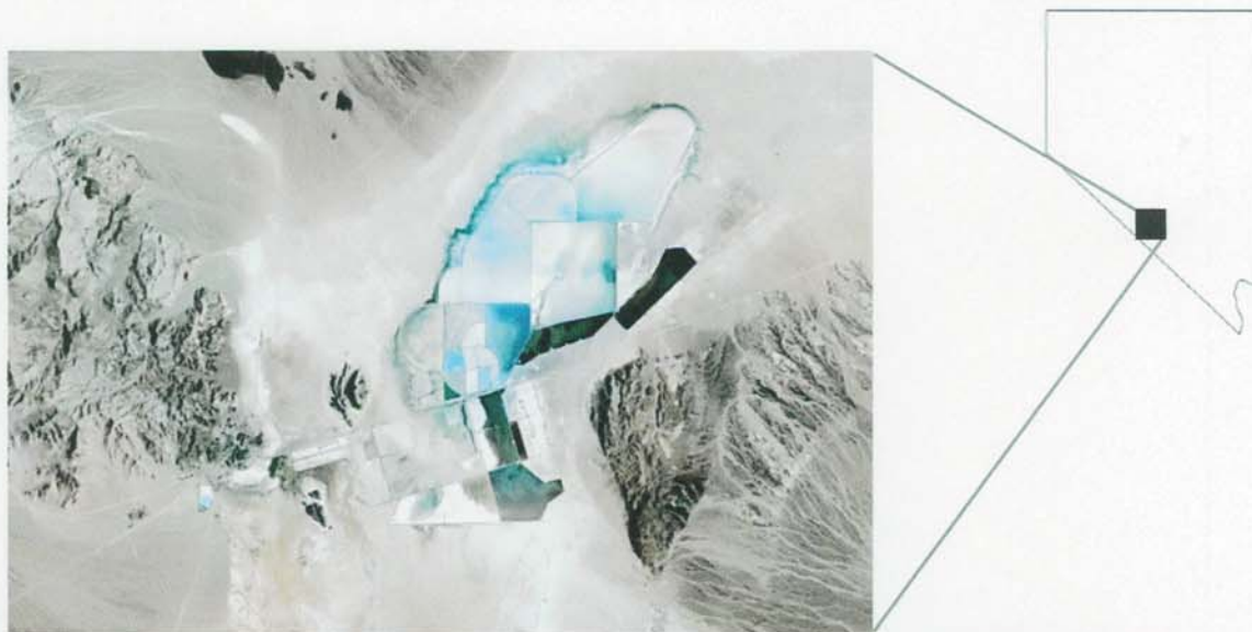
Figure 1. USDA Farm Service image of Clayton Valley. The town of Silver Peak is on the left, with evaporation ponds for lithium ore concentration on the right. Clayton Valley is located in Esmeralda County in Nevada near the border with California. Image taken directly from Google Earth.
