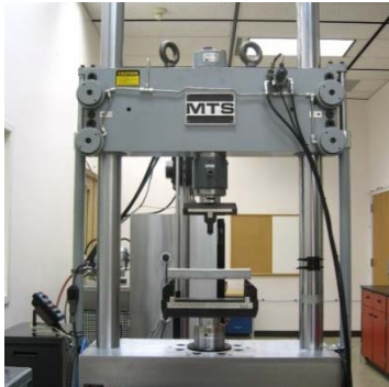
Figure 2 The MTS Universal Test Machine (UAA SOE) used to determine rod tensile properties
