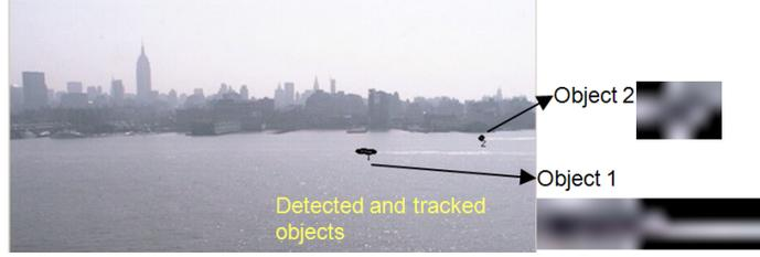
**Fig. 3.** (Left) A sample frame from the surveillance video with two tracked objects. (Right) The tracked objects' background subtraction-based representations; the histograms of these representations are the feature vectors of the objects in this frame.
